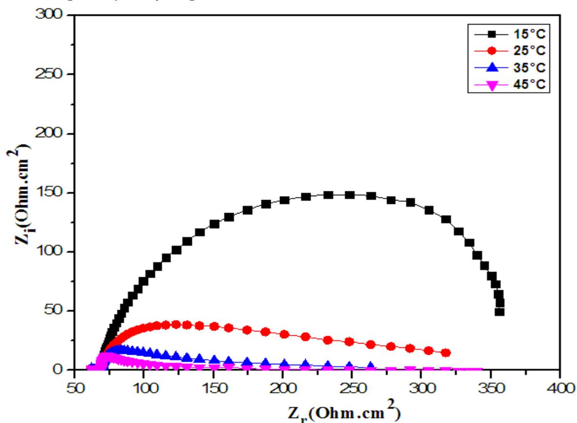
**Figure 7.** Nyquist curves of aluminum in 0.1 M Na<sub>2</sub>CO<sub>3</sub> without inhibitor at different temperatures.
