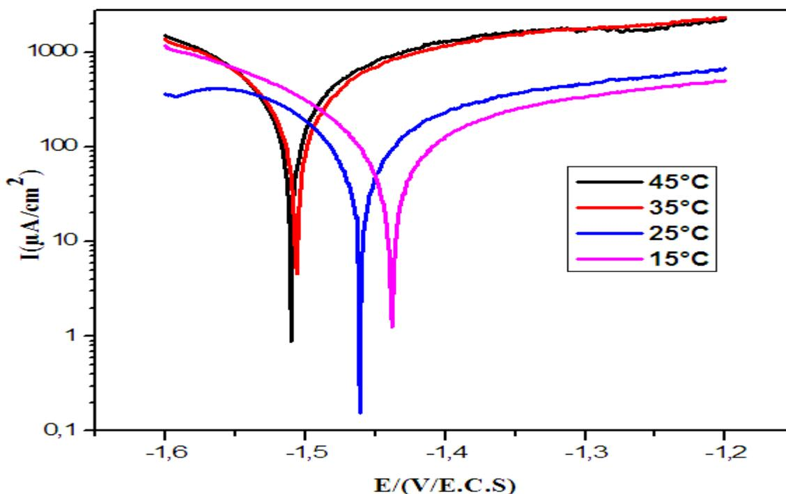
**Figure 5.** Polarization curves of aluminum in 0.1 M  $\text{Na}_2\text{CO}_3$  without inhibitor at different temperatures.
