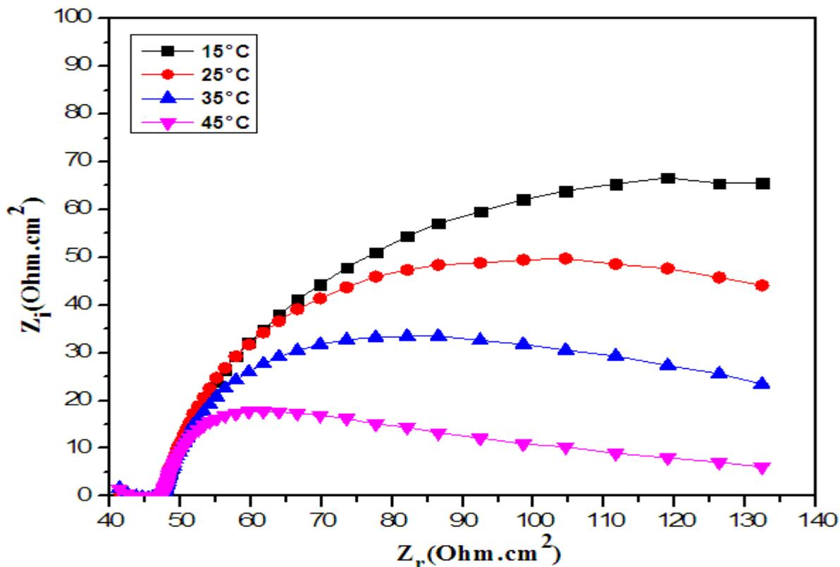
**Figure 8.** Nyquist curves of aluminum in 0.1 M Na<sub>2</sub>CO<sub>3</sub> with 1600 ppm of the inhibitor at different temperatures.
