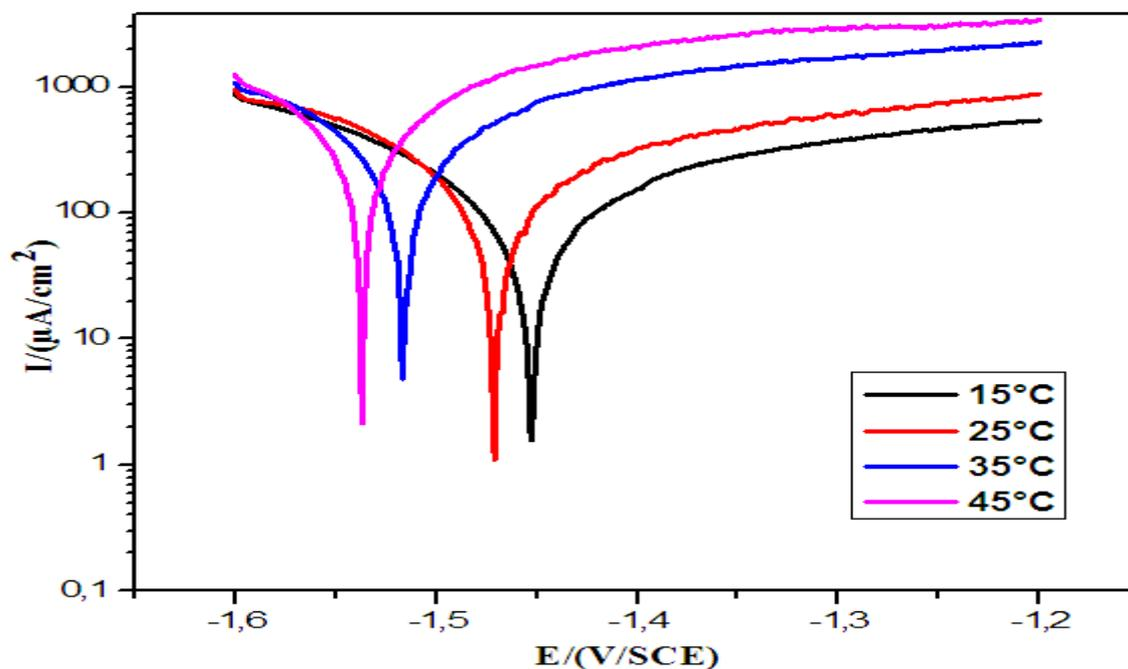
**Figure 6.** Polarization curves of aluminum in 0.1 M  $\text{Na}_2\text{CO}_3$  with the presence of 1600 ppm of the inhibitor at different temperatures.
