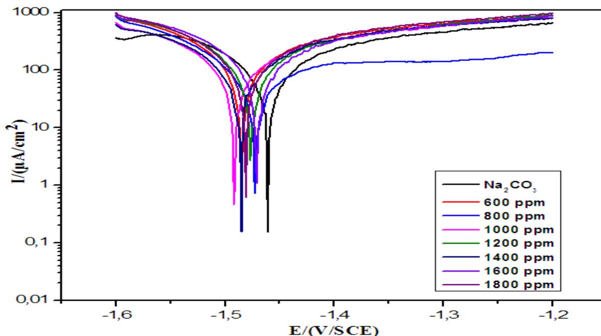
**Figure 2.** Polarization curves of aluminum in 0.1 M  $\text{Na}_2\text{CO}_3$  with and without inhibitor at  $25 \pm 0.1$  °C.
