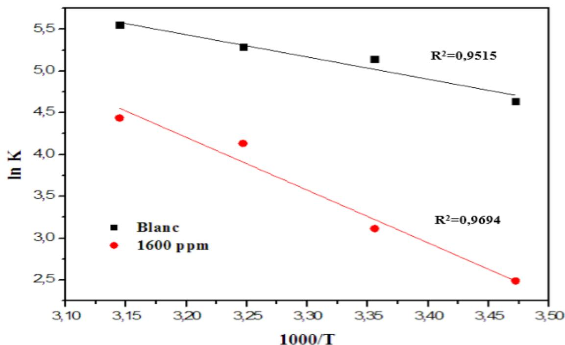
Figure 9. Arrhenius Curves of aluminum in 0.1 M  $\text{Na}_2\text{CO}_3$  with and without inhibitor
