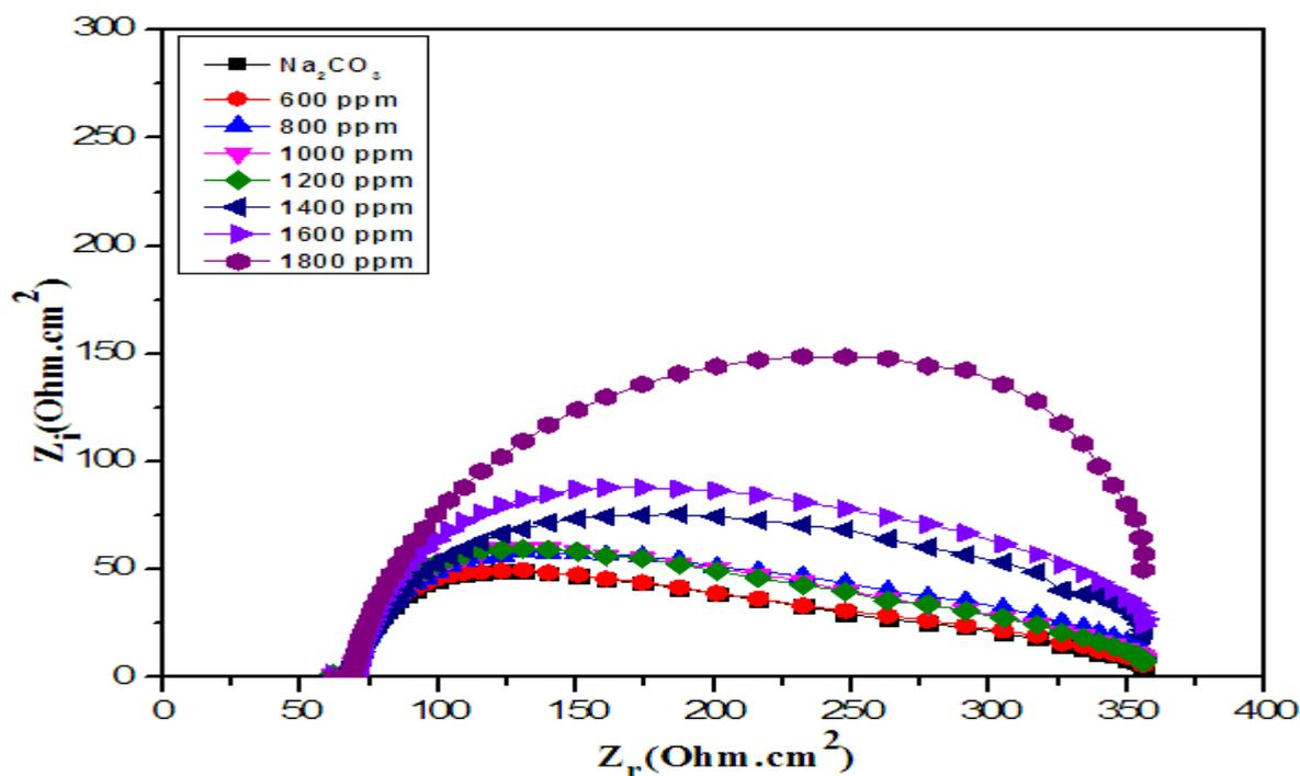
Figure 3. Nyquist curves of aluminum in  $\text{Na}_2\text{CO}_3$  with and without addition of the inhibitor at  $25 \pm 0.1$  °C.
